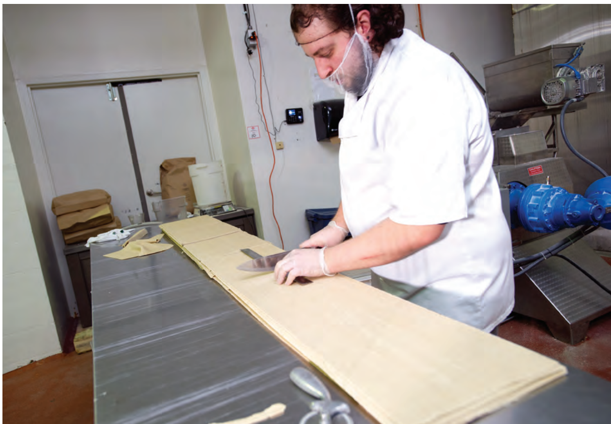
A Gabriella's Kitchen production team member cuts the thick layers of pasta dough produced on the Agnelli pasta-making machine into precisely-measured slabs to go inside a collator for repeated pressing into the desired thinness.
