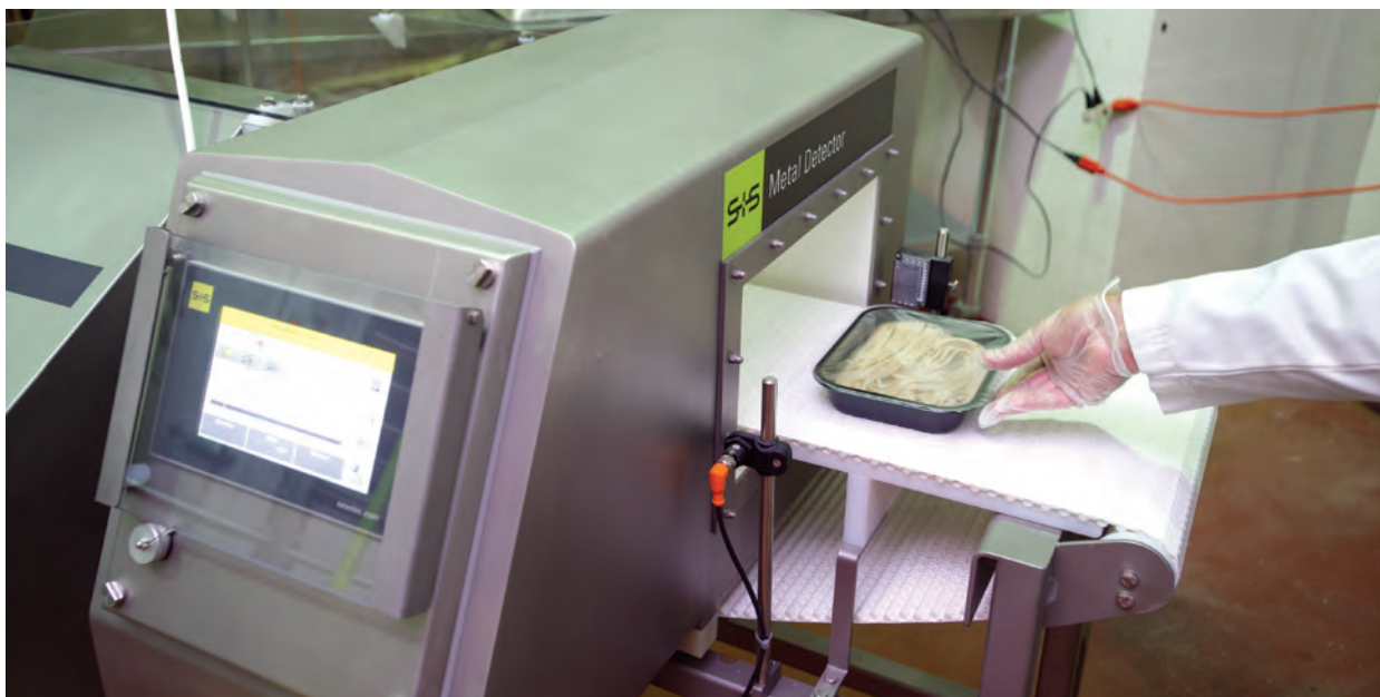
Sealed tray packages pass through a high-sensitivity quality assurance check by the plant’s S+S brand metal detection system, manufactured by Sesotec, sold by JG Packaging and installed by RJP Packaging.
