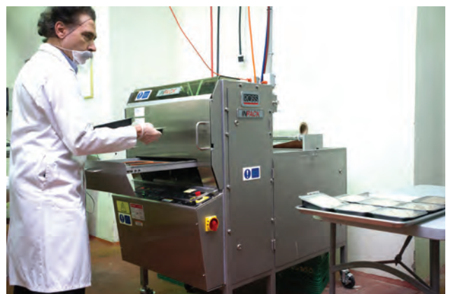
Depending on operator speed, the Ross Inpack tray-sealer can produce from eight to 12 finished packs per minute.
