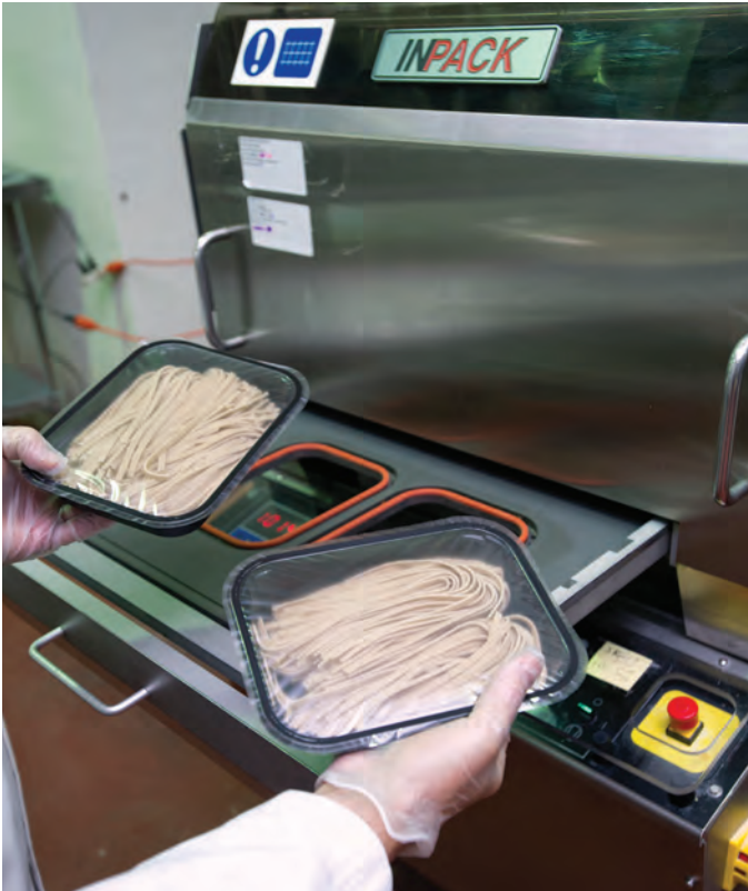
The Ross Inpack tray-sealer distributed by Reiser produces two gas-flushed, fully-sealed tray packages per cycle.
