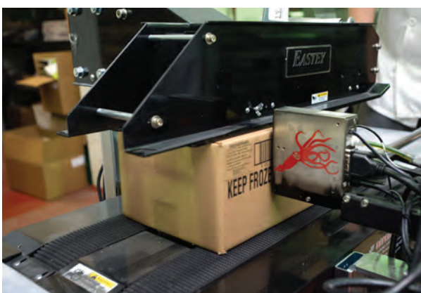
Model CO Pilot 382 case-coder springs into action to apply product barcode and other graphics onto the loaded carton. A close-up of the broad range of character sizes and fonts produced by Squid Ink's model CO Pilot 382 case-coder.
