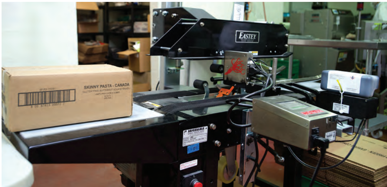
A semi-automatic Eastey case-sealer is positioned close to the Squid Ink case-coder in order to make optimal use of Gabriella's Kitchen's very limited available space to take care of all the necessary secondary packaging requirements.
