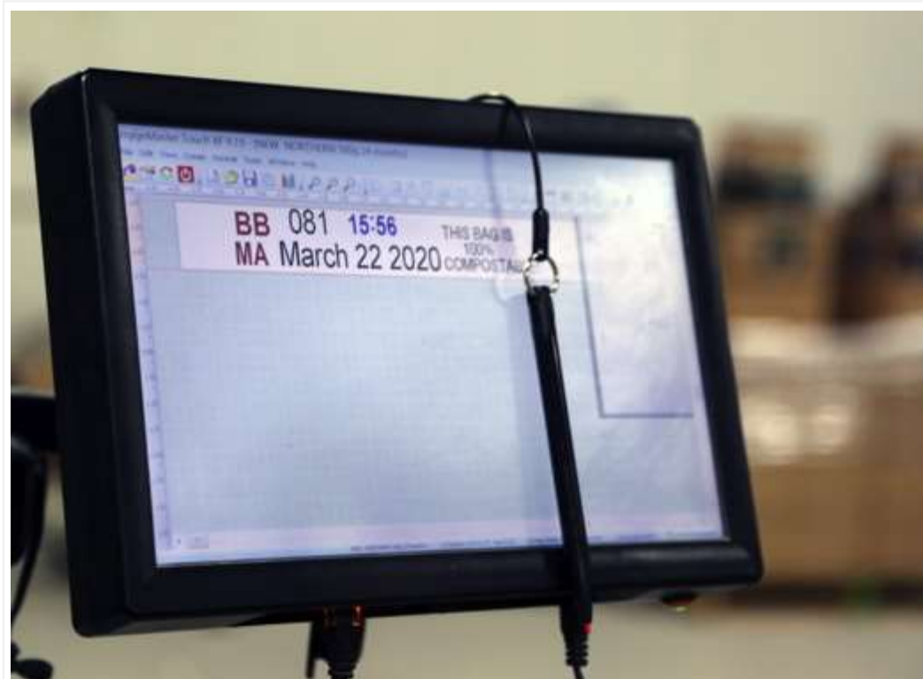
A controller for the Squid Ink AutoPilot, sold via Dependable Marking Systems, shows the type of data to applied via the coder to product packaging: time of manufacture, a four-year best-before date, lot code data, and a message indicating that the bag is 100 percent compostable.
