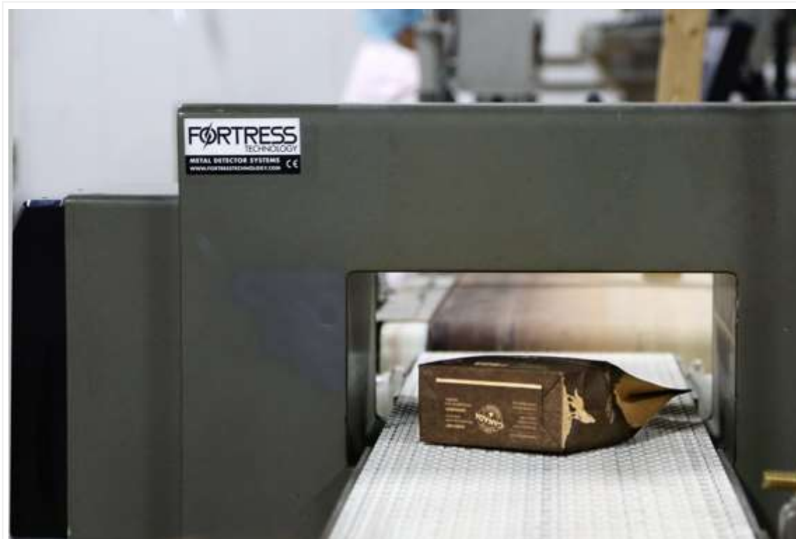
The bakery uses a Stealth metal detection unit manufactured by Fortress Technology, providing Northern Pet Products with an additional comfort level regarding the safety of its healthy dog biscuits, thanks to the system's highly-sensitive digital signal processing tech. (Below) A view of the Stealth's control panel.
