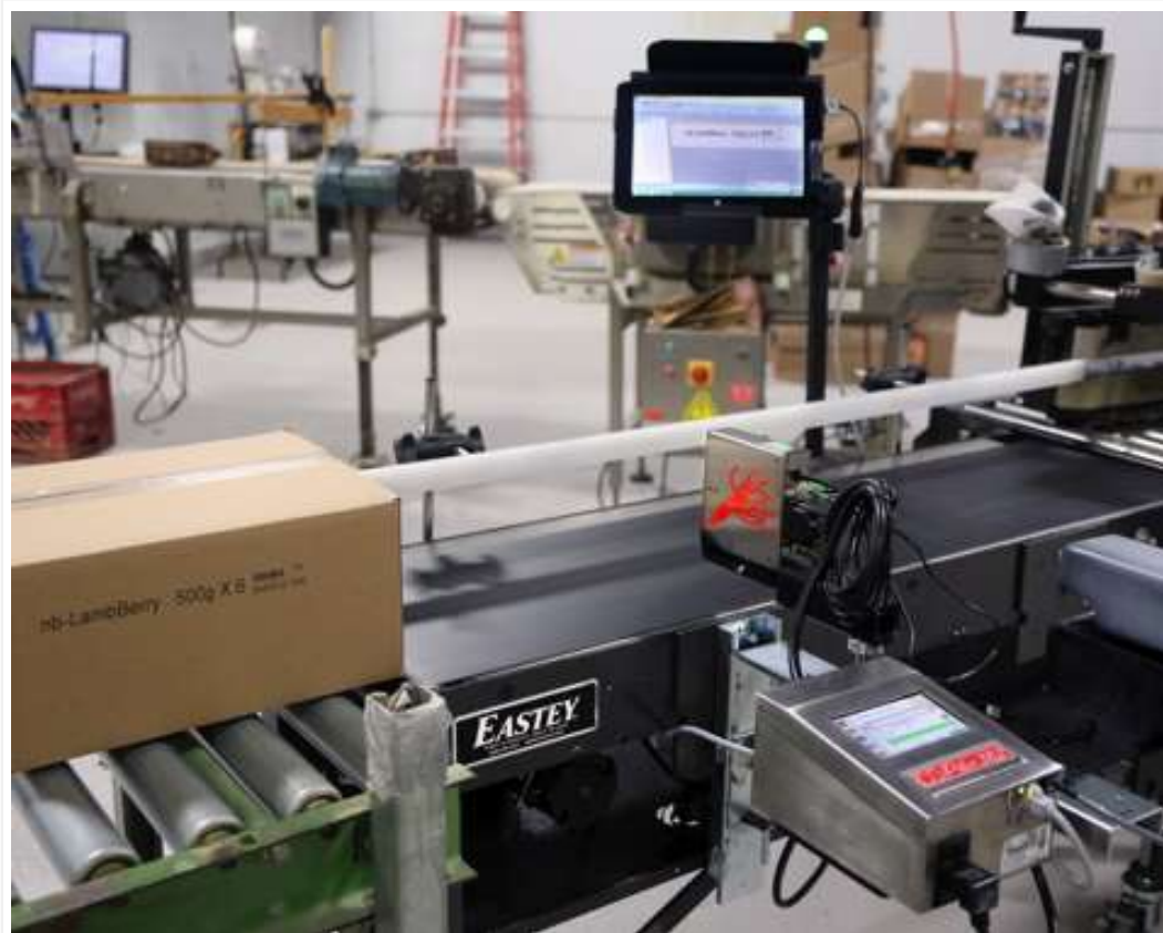
A CoPilot 382 manufactured by Squid Ink is mounted on an EasteY EC1248 conveyor applying product identification data after exiting an EasteY SB-2 Taper unit, which were all supplied to Northern Pet Products by Dependable Marking Systems.
